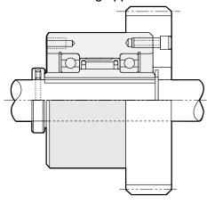
The FRB Series is a special design clutch, suitable for both low-speed driving and high speed overrunning and back-stopping applications.
