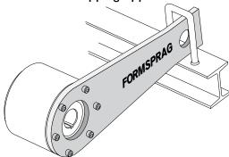
The FRB clutch must be secured to the shaft by customer supplied snap-ring, set collar, spacer, etc, in order to provide axial restraint.
