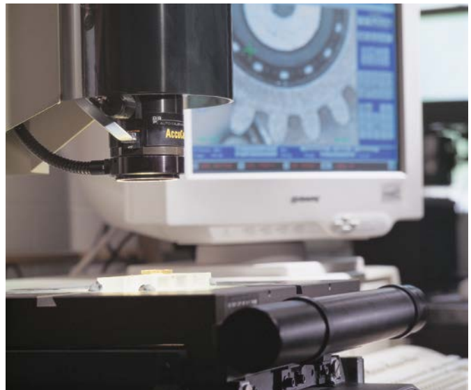
A vision system quickly verifies print conformance.
