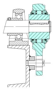
Fig. 5a: Installation example RSBW
