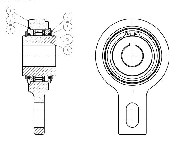
Fig. 1 Structure of one-way clutch RSBW
