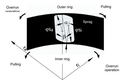
Fig. 2 Pulling/Overrun operation
