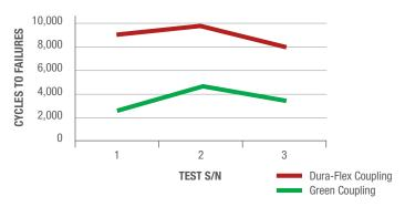
When a new, out-of-the-box, Dura-Flex coupling and a green coupling were subjected to a stop-start cycle test, Dura-Flex was 2X –100X better.
