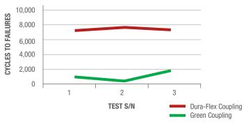
Dura-Flex outlasted the competitor in the cycle testing with up to 2 degrees of shaft misalignment.
