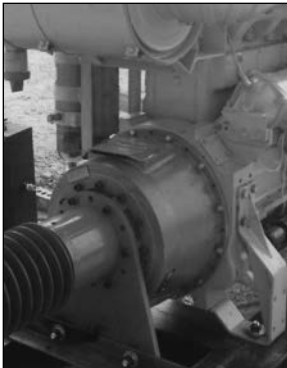
Wichita PTO mounted on Caterpillar diesel engine.
